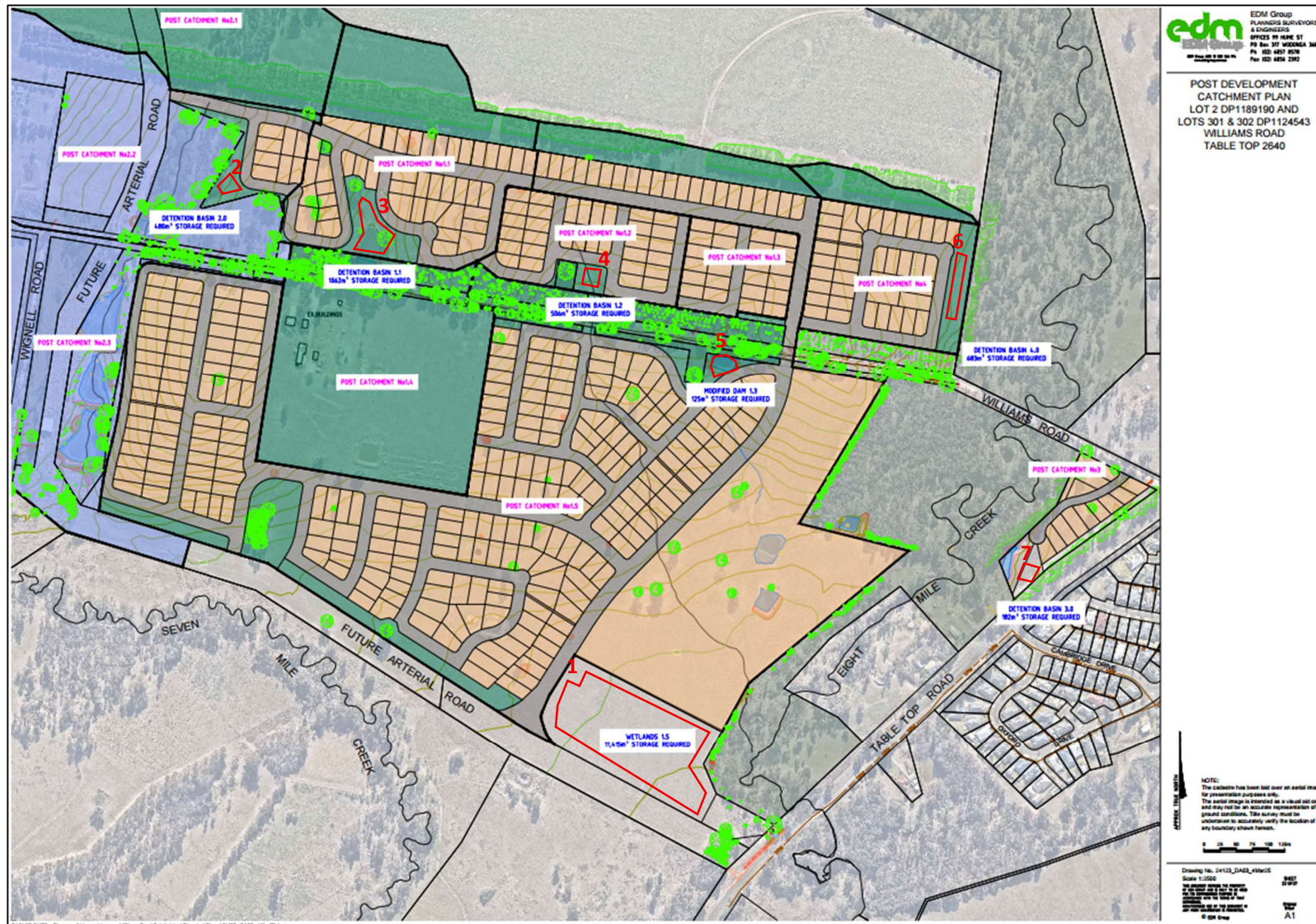
Figure 6: Catchment plan (post development) showing locations of 6 stormwater detention basins and wetland (red polygons) (Source: EDM Designs 2025)
